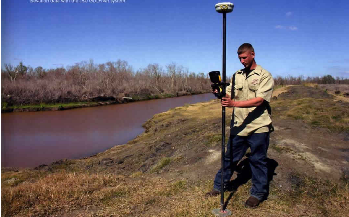
T. Baker Smith field technician Brody Davis takes elevation data with the LSU GULFNet system.
